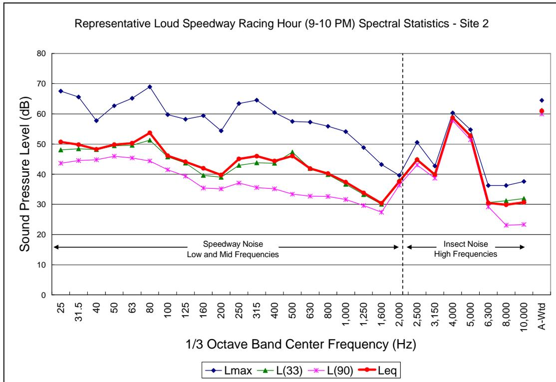
**Figure 4:** Example Frequency Spectrum of Speedway Measurements Illustrating Insect Noise
