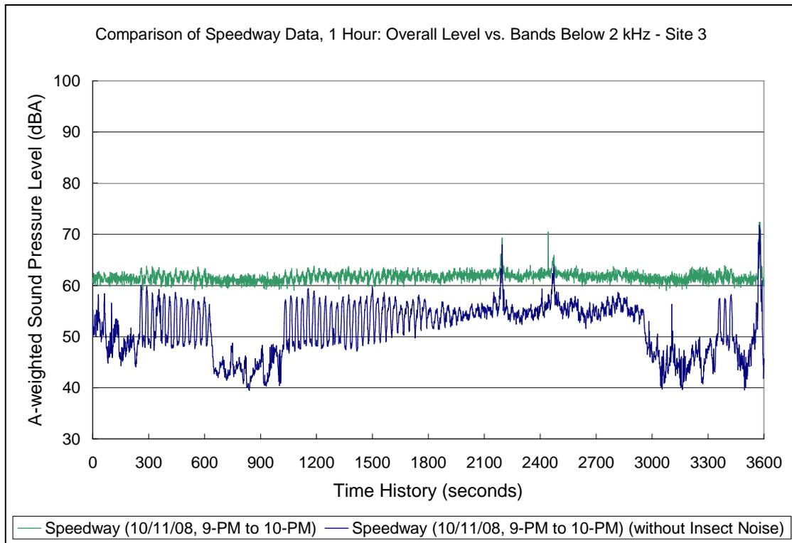
**Figure 5:** One Hour Example Comparison of Speedway Measurements: Overall Level vs. Bands Below 2 kHz
