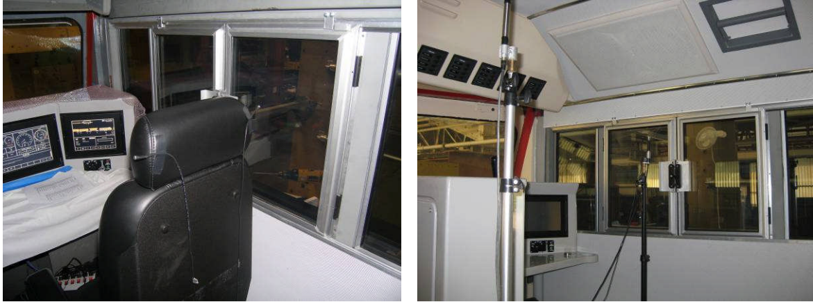
Figure 4: Error Microphones on Seat and Control Loudspeaker in Ceiling
