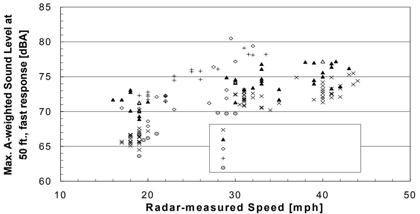
Figure 5. A-weighted Sound Levels of Snow Vehicles versus Speed
