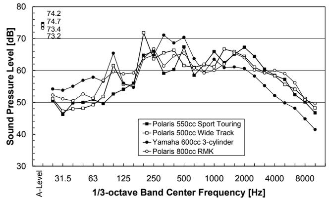
Figure 7. Sound Level Spectra of 2-Stroke Snowmobiles at 30 to 35 mph
