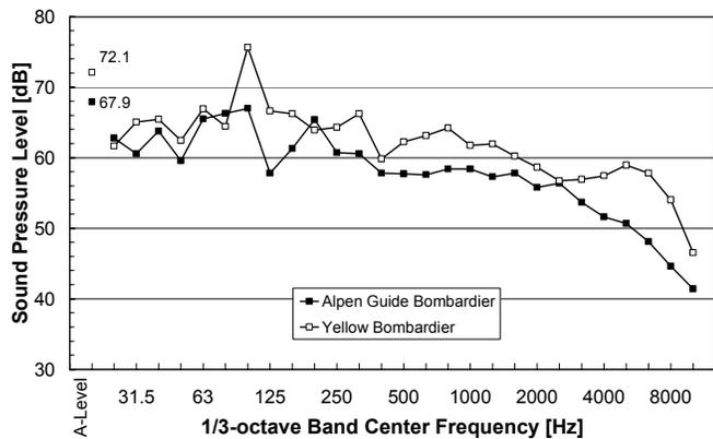
**Figure 9. Sound Level Spectra of Bombardier Snow Coaches at 20 mph**
