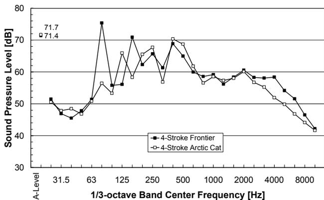
Figure 6. Sound Level Spectra of 4-Stroke Snowmobiles at 30 to 35 mph
