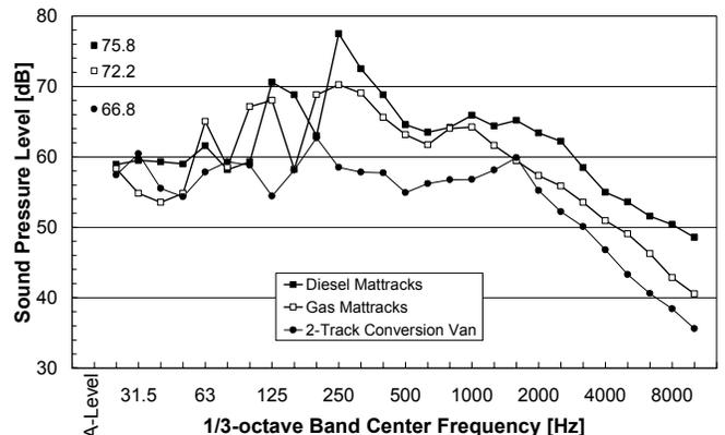
Figure 8. Sound Level Spectra of 4-track and 2-track Snow Coaches at 20 mph
