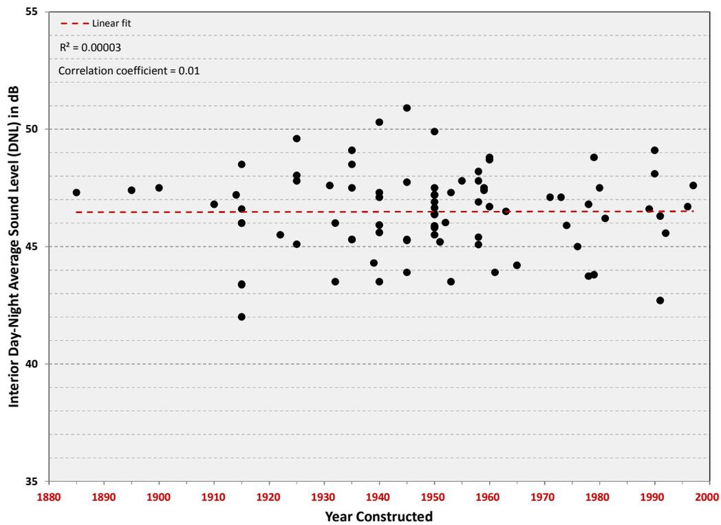
Figure 8: Aircraft Interior DNL vs Single-Family Residence Year Constructed
