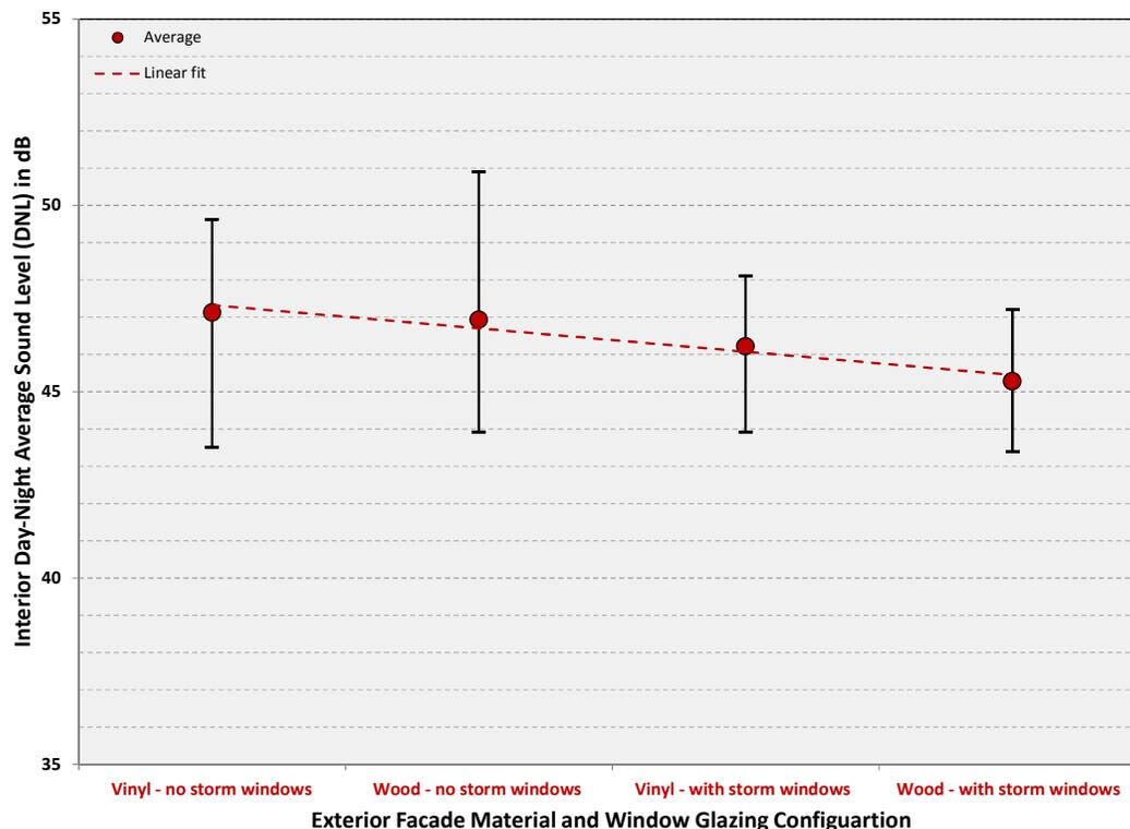
**Figure 13:** Range of Aircraft Interior DNL by Single-Family Residence Facade Material and Window Configuration
