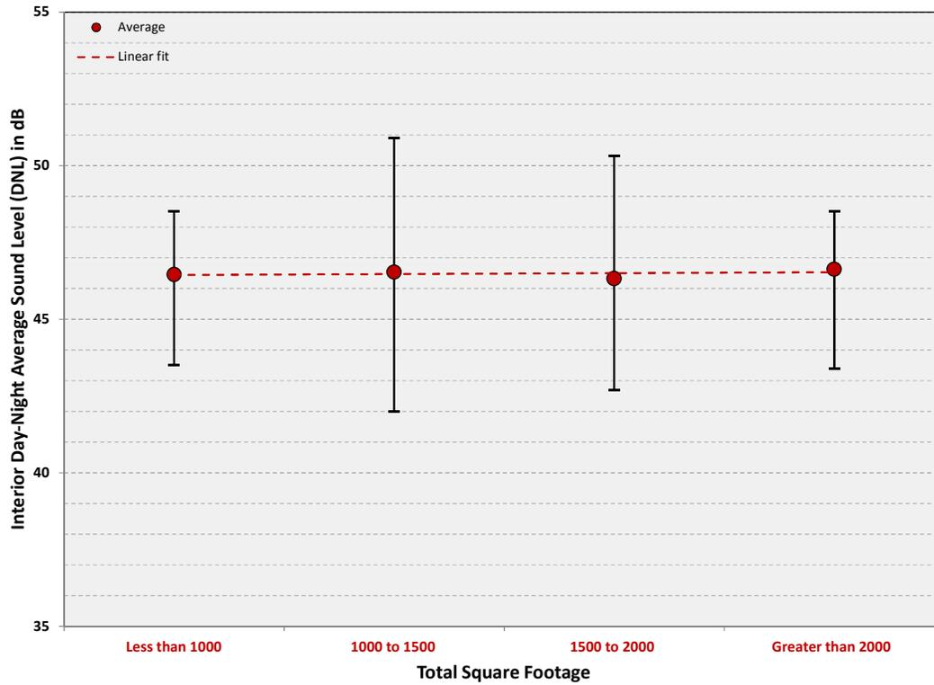
**Figure 5:** Range of Aircraft Interior DNL by Single-Family Residence Total Square Footage ( $1.00 \text{ ft}^2 = 0.09 \text{ m}^2$  and  $1.00 \text{ m}^2 = 10.76 \text{ ft}^2$ )
