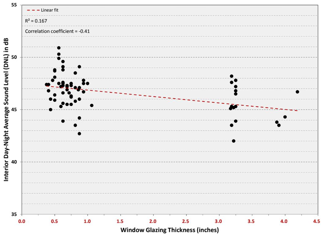
Figure 12: Aircraft Interior DNL vs Single-Family Residence Window Glazing Thickness (1.00 in = 2.54 cm and 1.00 cm = 0.39 in)
