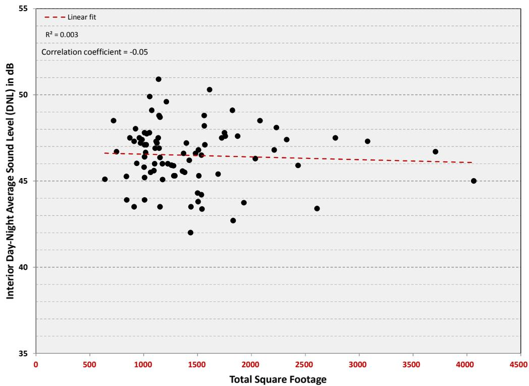
**Figure 6:** Aircraft Interior DNL vs Single-Family Residence Total Square Footage ( $1.00 \text{ ft}^2 = 0.09 \text{ m}^2$  and  $1.00 \text{ m}^2 = 10.76 \text{ ft}^2$ )
