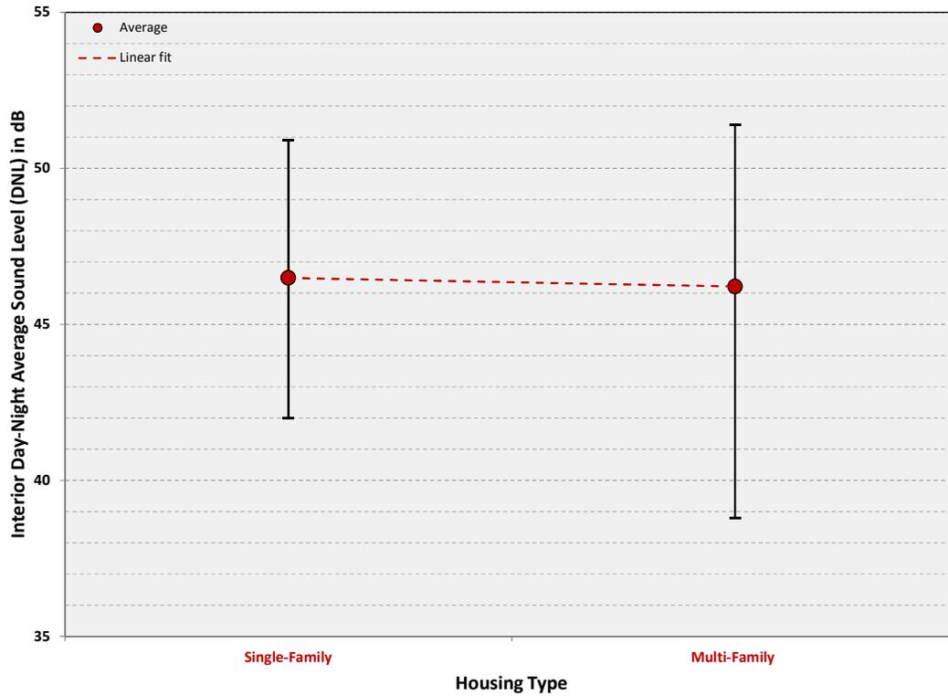
Figure 1: Range of Aircraft Interior DNL by Residential Housing Type
