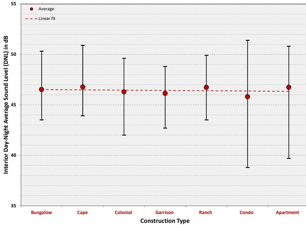
Figure 3: Range of Aircraft Interior DNL by Residential Construction Type
