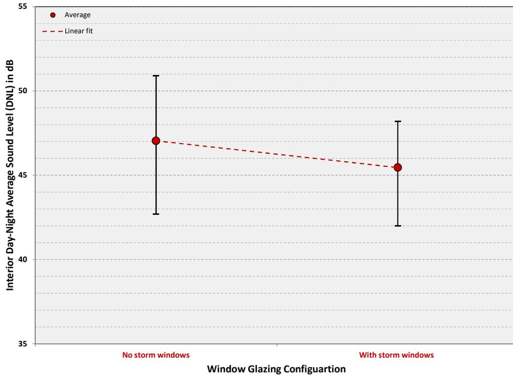
Figure 11: Range of Aircraft Interior DNL by Single-Family Residence Window Configuration
