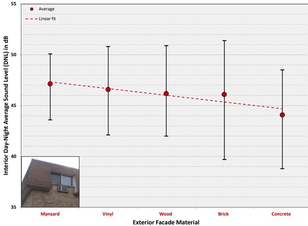
Figure 9: Range of Aircraft Interior DNL by Residential Exterior Facade Material
