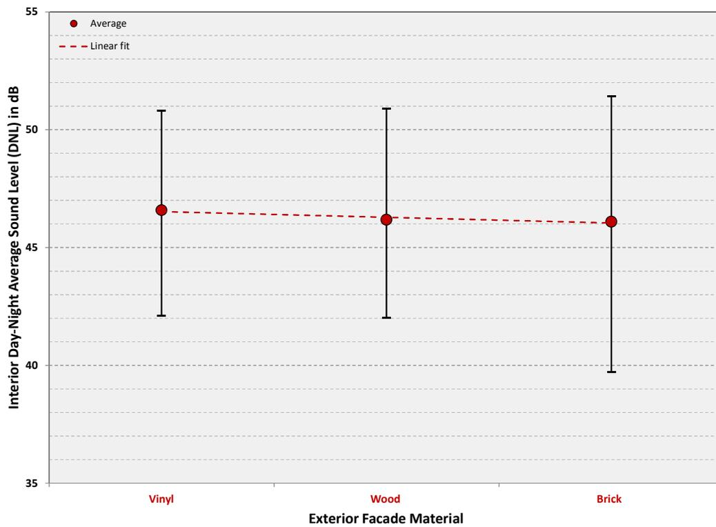
Figure 10: Range of Aircraft Interior DNL by Most Typical Residential Facade Materials
